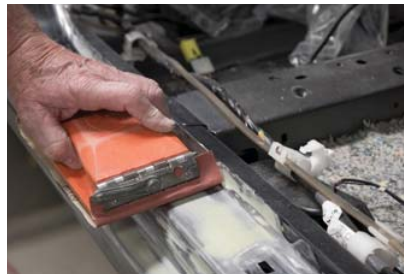
Off-hand grinding - Bodywork
